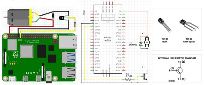
(Transistor numbering (1,2,3) in the above sketch is unusual, a limitation of the RPi fzbz I used) From top to bottom in the picture and diagram it should be:
